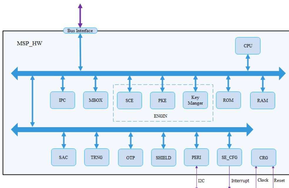
TOE and other system via Bus interface, Bus interface will connect the inner of the TOE to SOC.
